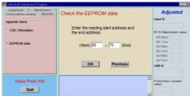
Figure 5-54. Reading Start/End Address Input
