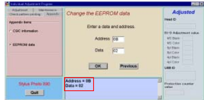
Figure 5-58. EEPROM Data Change Completed
