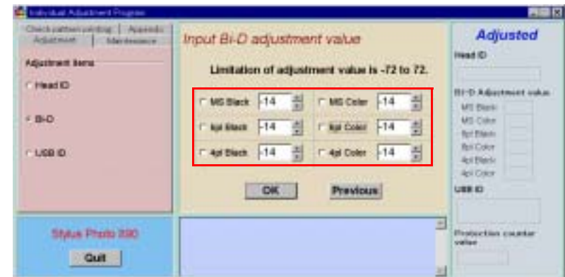
Figure 5-28. Input Bi-D Adjustment Value Window
