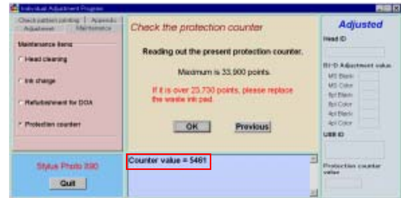
Figure 5-45. Protection Counter Value Displayed
