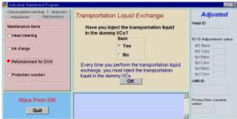
Figure 5-42. Transportation Liquid Exchange Window
