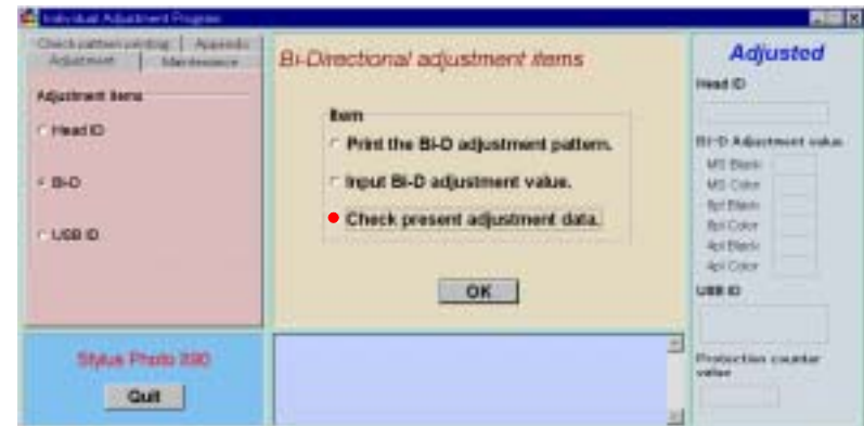
Figure 5-31. Bi-Directional Adjustment Window
