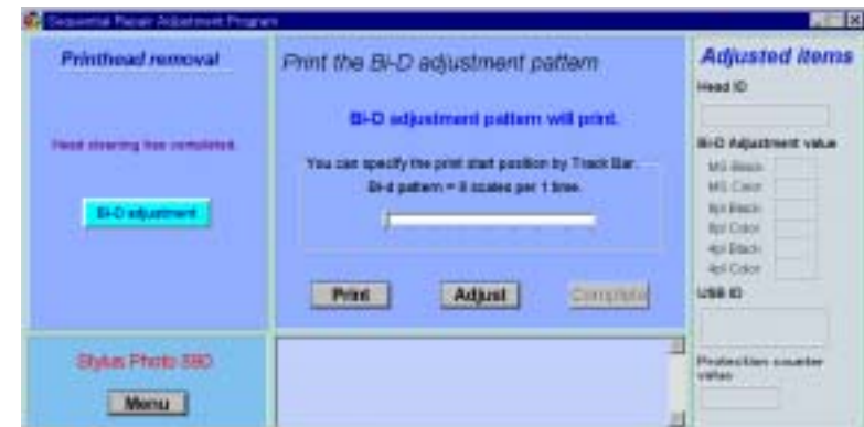
Figure 5-66. Bi-D Adjustment Pattern Printing
