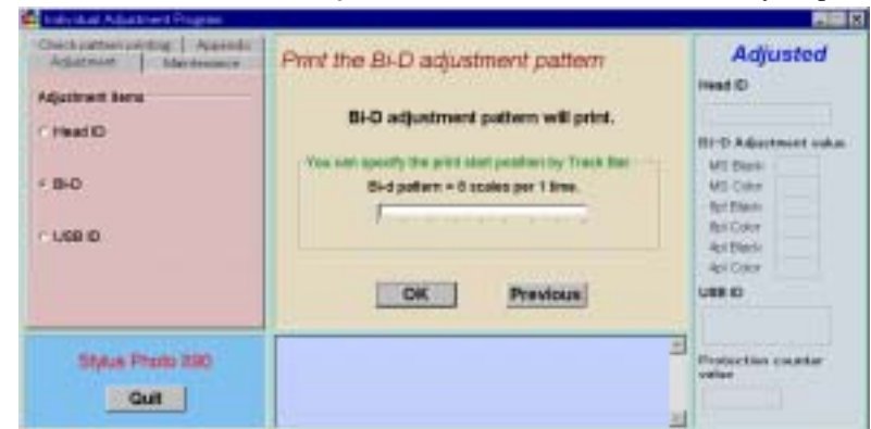
Figure 5-22. Bi-Directional Adjustment Pattern Printing
