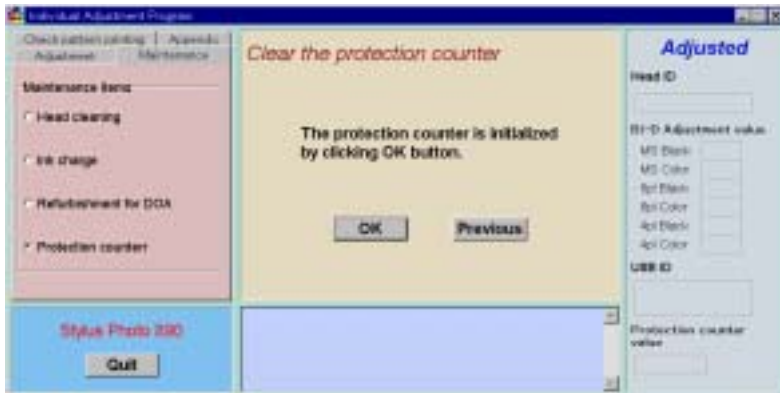
Figure 5-47. Clear the Protection Counter Window
