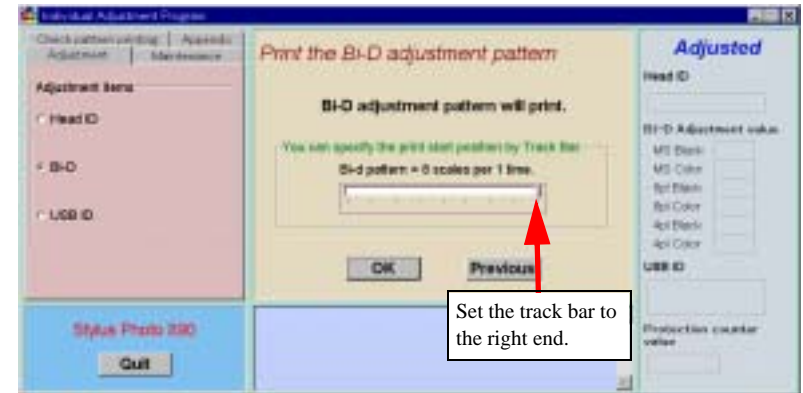
Figure 5-24. Second Bi-Directional Adjustment Pattern Printing
