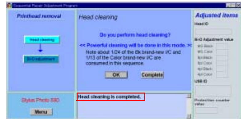
Figure 5-65. Head Cleaning Completed
