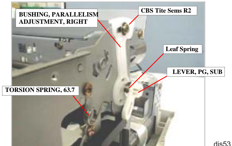
Figure 4-49. LEVER, PG, SUB Removal
