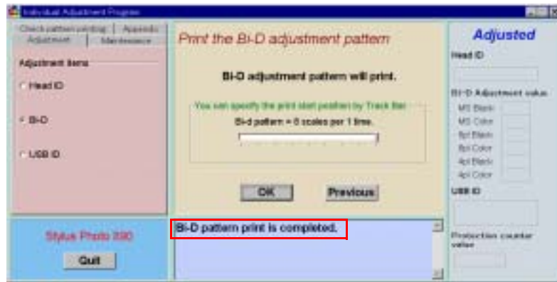
Figure 5-26. Bi-Directional Adjustment Pattern Printing Completed
