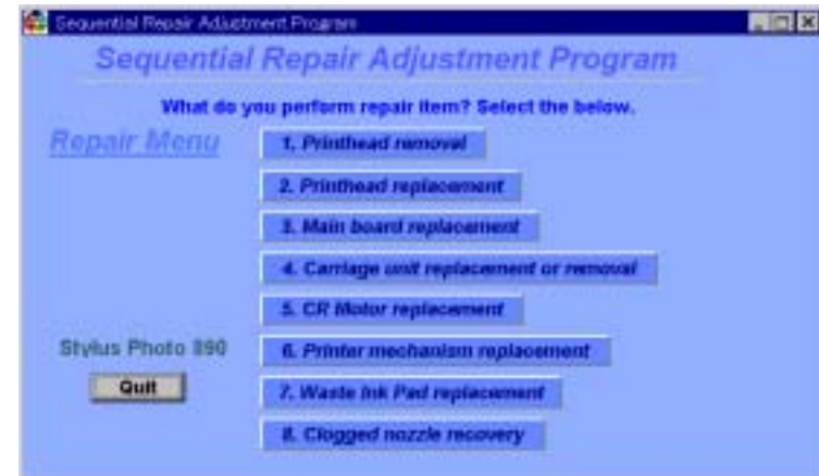
Figure 5-63. sequential Repair Adjustment Program Main Menu
